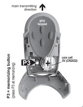
Range: The largest possible range results of an optimum installation of the receiver antenna, aimed transmission in direction of the receiver, free of obstacles, with high position of transmitter and actuation of transmitter button for at least 1-2 seconds
