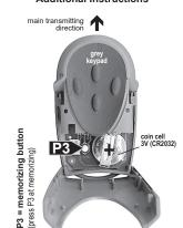
Range: The largest possible range results of an optimum installation of the receiver antenna, aimed transmission in direction of the receiver, free of obstacles, with high position of transmitter and actuation of transmitter button for at least 1-2 seconds.
