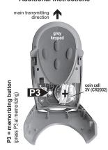
Range: The largest possible range results of an optimum installation of the receiver antenna, aimed transmission in direction of the receiver, free of obstacles, with high position of transmitter and actuation of transmitter button for at least 1-2 seconds
