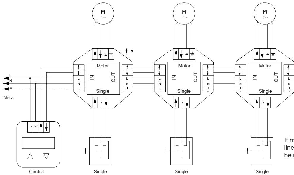
If more than 4 motors are connected to a line, a larger wire cross-section should be used.
