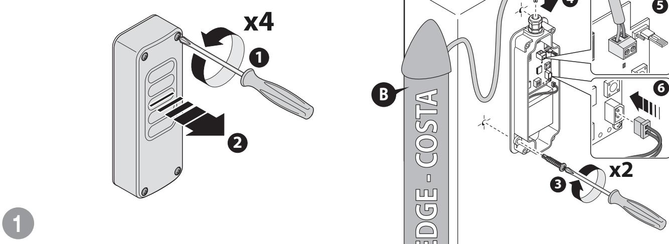
INSTALLAZIONE UNITÀ FISSA - STATIONARY UNIT INSTALLATION - INSTALLATION DE L'UNITÉ FIXE
