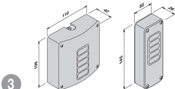
INTERFACCIA PER COSTA SENSIBILE, INTERFACE FOR THE SAFETY EDGE, INTERFACE POUR BORD DE SÉCURITÉ, TRANSCEIVER-SCHNITTSTELLE - INTERFAZ TRANSCPTOR
