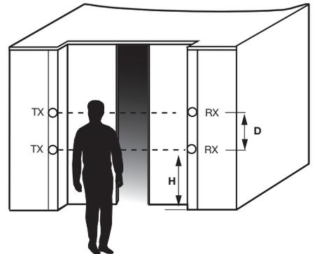
LA DISTANCE TX-RX NE DOIT PAS DÉPASSER LES 15 MÈTRES. LA DISTANCE "H" DÉPEND DE LA HAUTEUR DE LA PERSONNE OU DU MATÉRIEL QUI DOIT ÊTRE DÉTECTÉ.
