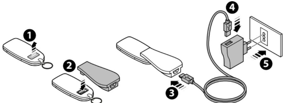
• CAMBIO BATTERIA • CHANGING THE BATTERY • REMplacement DE LA PILE
