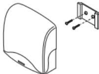
The outdoor receiver is fitted using "fast-fitting" brackets. After connecting the wiring the case should be slid onto the bracket therefore fixing it to the wall. If any repair work is necessary the case can be easily extracted by pushing upwards the action of which will separate it from the bracket.
